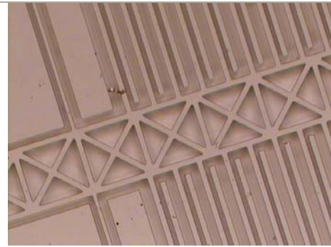
Figure 5: Image of MEMS GCA Test Article Showing the Central Beam Structure
