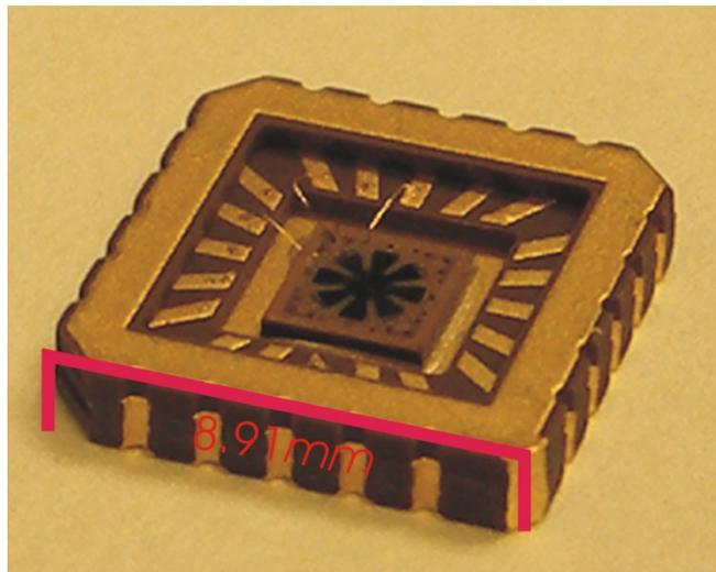
**Figure 8: Chip Carrier for Prototyping of MEMS Devices**
