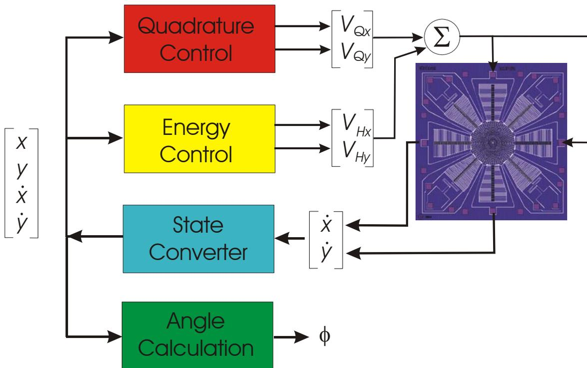
Figure 7: Overview of RIG Control System
