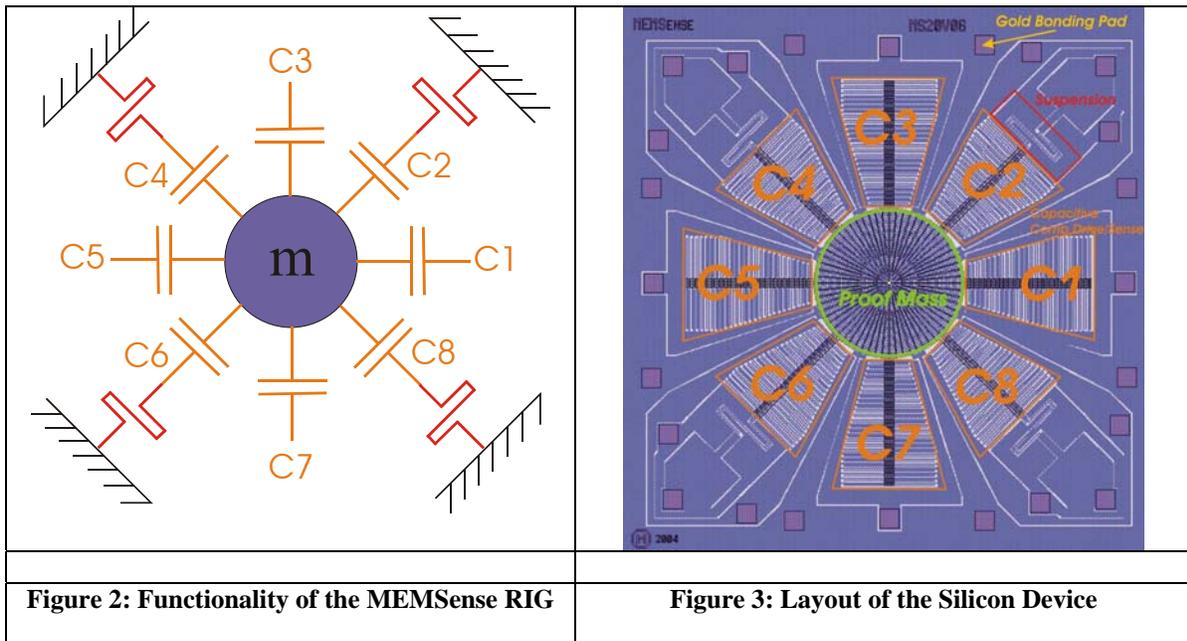
The silicon implementation has the functionality as shown in Figure 2. An example of a MEMSense design is shown in Figure 3. The capacitive elements are constructed from numerous interdigitated combs. Some typical values for candidate MEMS devices can be found in
