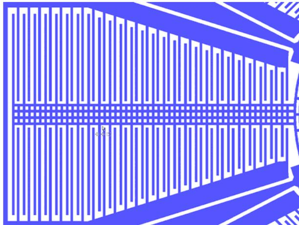
**Figure 5: Capacitive Comb Drive**
